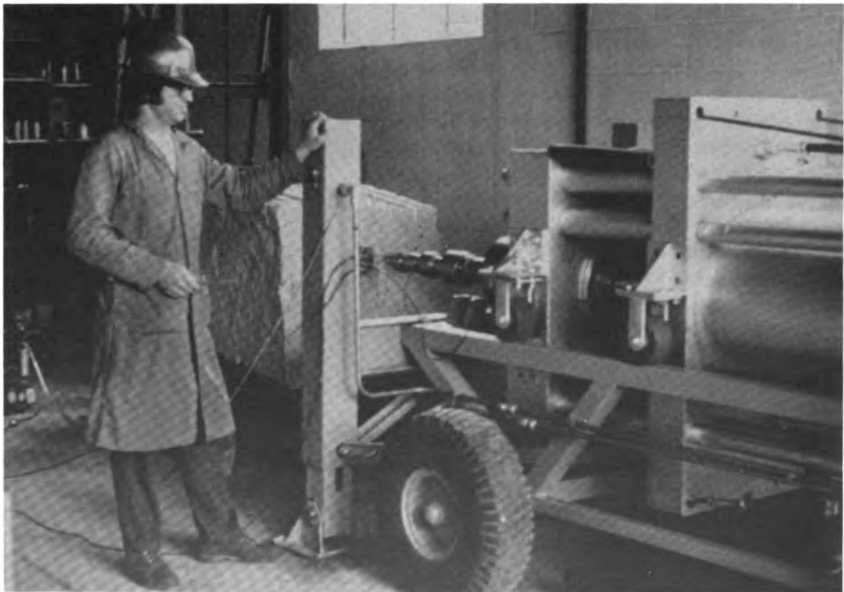
Figure 30. High Pressure Water Cannon Being Tested on Rock Test Cube.
