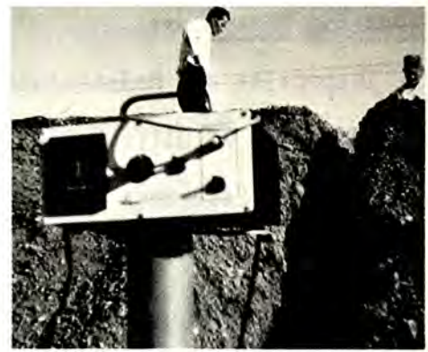
NULL INDICATOR USED FOR FINAL INSTALLATION CALIBRATION OF ALL ENBANKMENT DISPLACEMENT TRANSDUCERS
