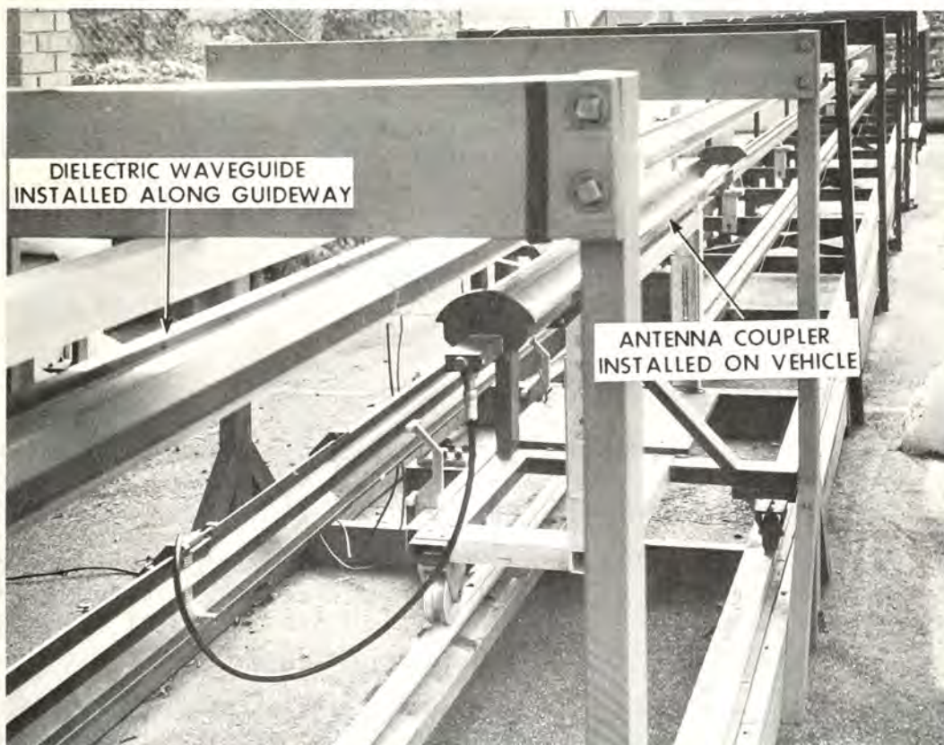
Dielectric Waveguide Laboratory Experiment for Communication Systems.
