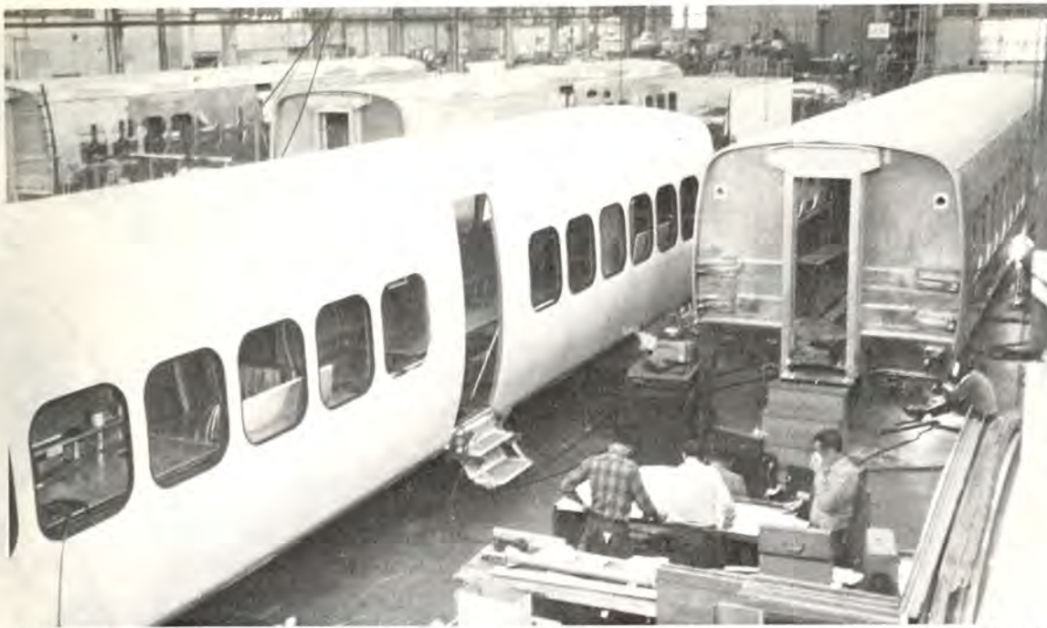
New Turbo Train Intermediate Cars Being Manufactured at United Aircraft Corporation (Two to be added to each trainset).
