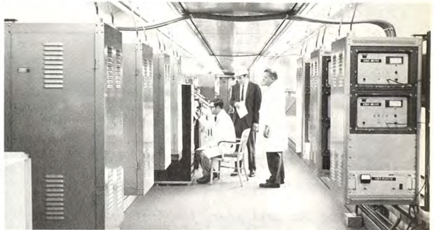
TRACK MEASUREMENT DATA RECORDING SYSTEM IN ONE OF THE RAIL RESEARCH TEST CARS
