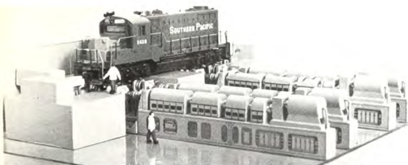
SCALE MODEL OF THE WHEEL-RAIL DYNAMICS SIMULATOR
