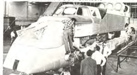
MATING OF BODY PRIMARY STRUCTURE WITH AIR DUCT CHASSIS
