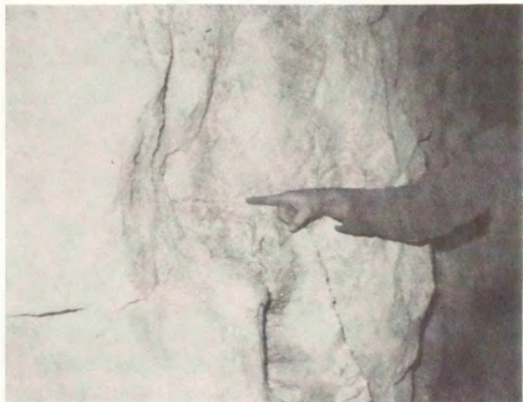
Figure 43a .Dolomitic Limestone Rock Face after 18 Water Jet Pulses at Jet Pressures Near 450,000 Pounds per Square Inch.
