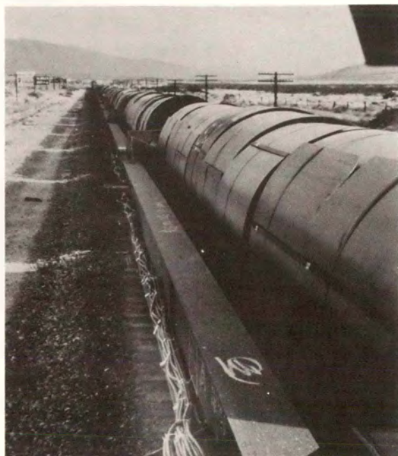
Figure 29a. Partial View of 52-Car Steel-Coil Unit Train, Showing the Cabling Connecting the Instrumentation Located throughout the Train to the FRA Digital Data Acquisition System.
