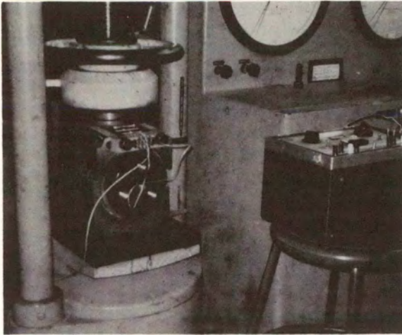
a. Laboratory Calibration of Truck Bearing Adaptor Sensors.
