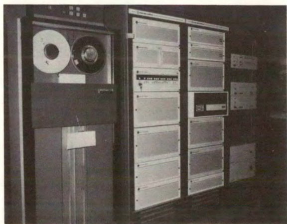
Figure 26. Profile Generator System Computer with Analog Conversion Equipment on the Right and Magnetic Tape Unit on the Left.
