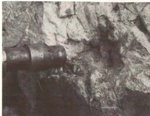
Figure 43b. Granite Gneiss Rock Face after 22 Water Jet Pulses at Jet Pressures Near 450,000 Pounds per Square Inch.
