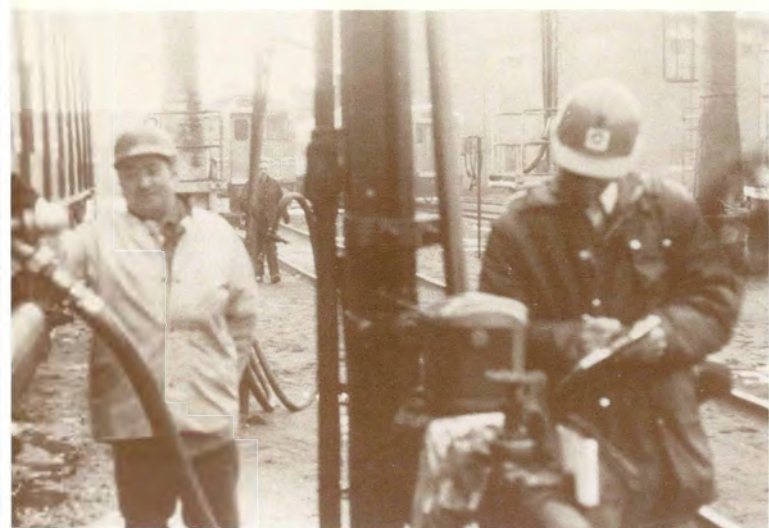
Figure 1. Research technician from the Transportation Systems Center records fueling of a diesel-electric locomotive during the conduct of fuel consumption measurements of various train operations.
