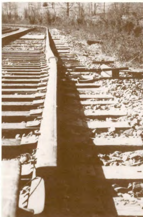
Figure 26. Maximum Distortion of the Concrete Tie Panel in the Chessie Tests at Sabot. Note Curved Alignments of Rail Indicating Superior Resistance of Concrete Ties to Lateral Displacement.
