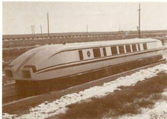
Figure 40. Prototype Tracked Air Cushion Vehicle (PTACV) on Test Track at TTC, Pueblo, Colorado.
