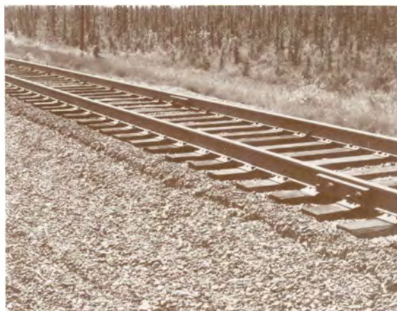
Figure 29. Ballast Shoulder Slump in the Houston Test of the Alaska Railroad.
