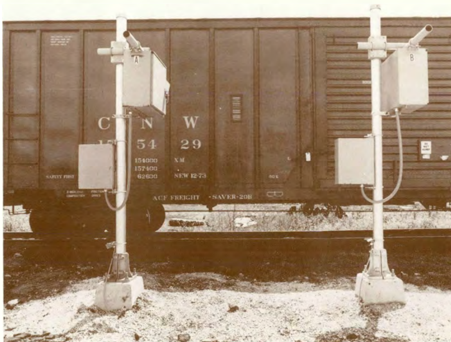
Figure 5. Two ACI test scanners reading ACI label on passing freight car. Five thousand cars passed the test site during the evaluation.
