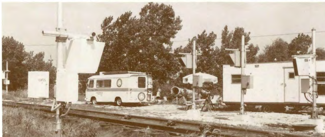
Figure 4. Test site (Proviso Yard, East-Chicago) used to evaluate potential improvements that can be made to increase the readability of optical automatic car identification (ACI) labels. One conventional scanner (left background) was compared to two improved scanners (foreground) from each of the two scanner suppliers. Data collection equipment was housed in trailer and motor van.
